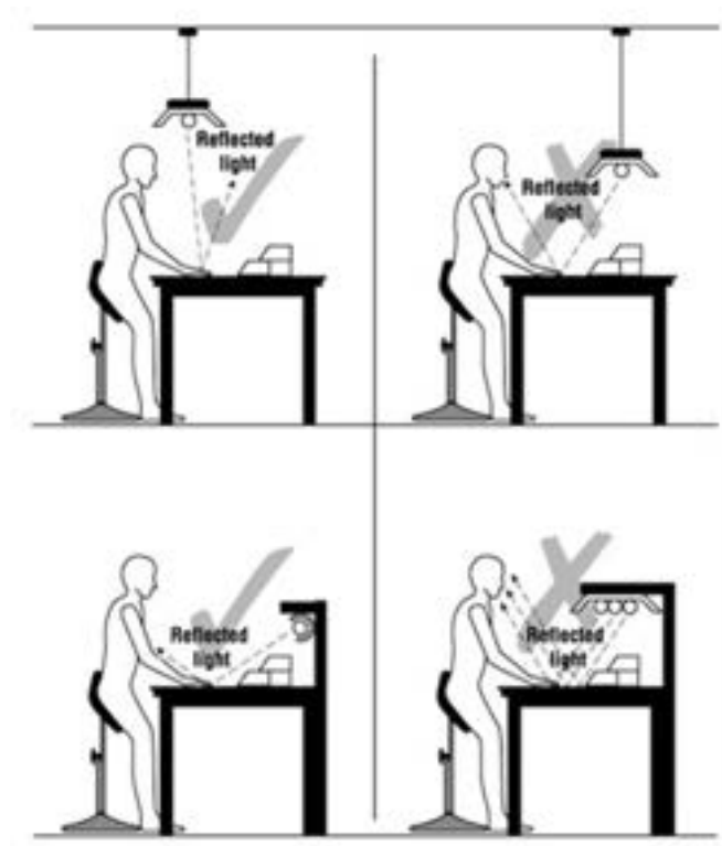
Figure 2.9: Poor lighting and elimination of glare
