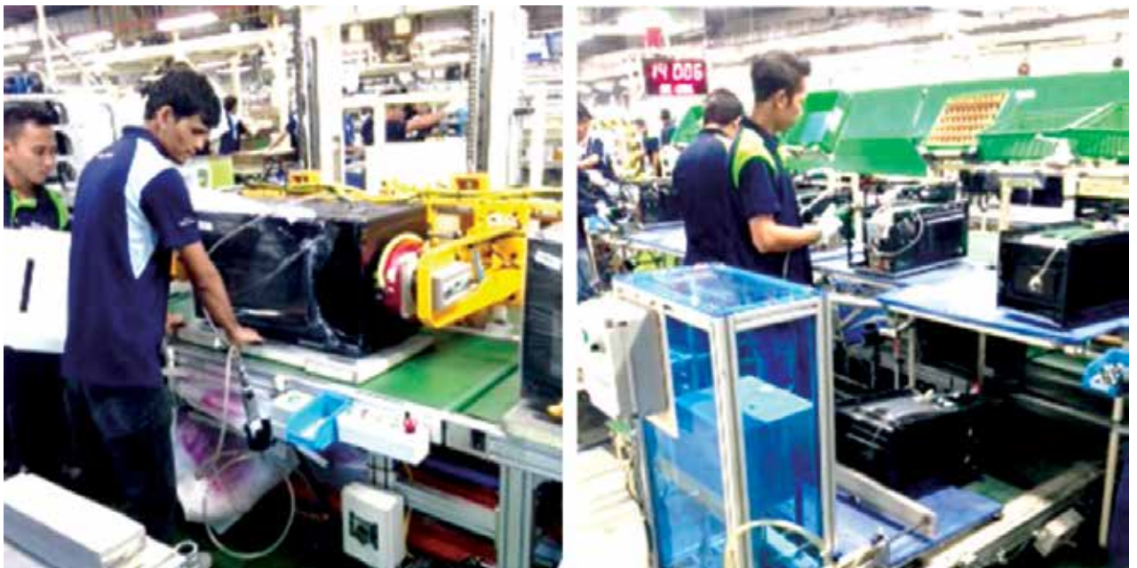
Figure 6.4: Auto-clamping lifter used to lift up/down and turn products (Left) and a hydraulic-cylinder lifter allows products to be lowered and pushed into transferring conveyor by means of a foot-switch (Right).
