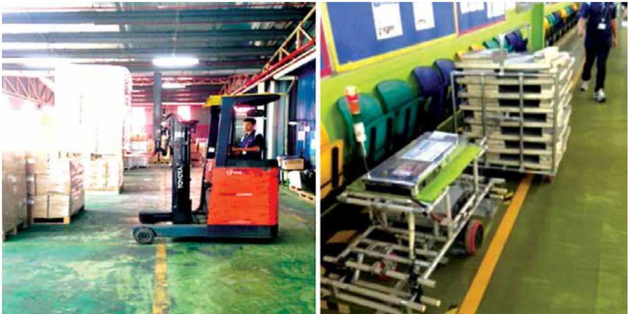
Figure 6.5: A powered-reach truck is used to move and lift materials short/long distances (Left). A tugging AGV used for pulling trolleys loaded with heavy objects between workstations (Right)
