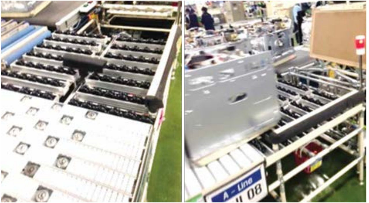
Figure 6.3: An assembly line embedded with roller tracks and ball bearings allows heavy objects to be turned and repositioned
