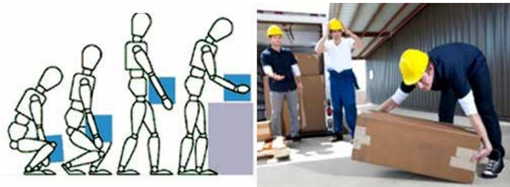
Figure 2.10: Correct lifting vs incorrect lifting technique
